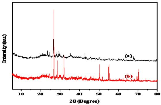
Figure 2. Powder XRD pattern of (a) pure and (b) Coumarin doped BTCC crystal
